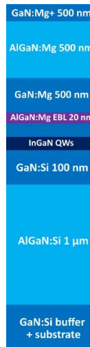
Fig. S1 : Epitaxial structure of the laser diode.
