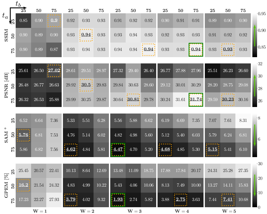
Fig. 4. Reconstruction performance analysis by varying t_a , t_b , and W for the spectral videos used in the experiments section 3 (see Visualization 1). Here, the optimal result for each heatmap is highlighted with a dotted orange square. Additionally, the better result per metric is highlighted with a straight green square.
